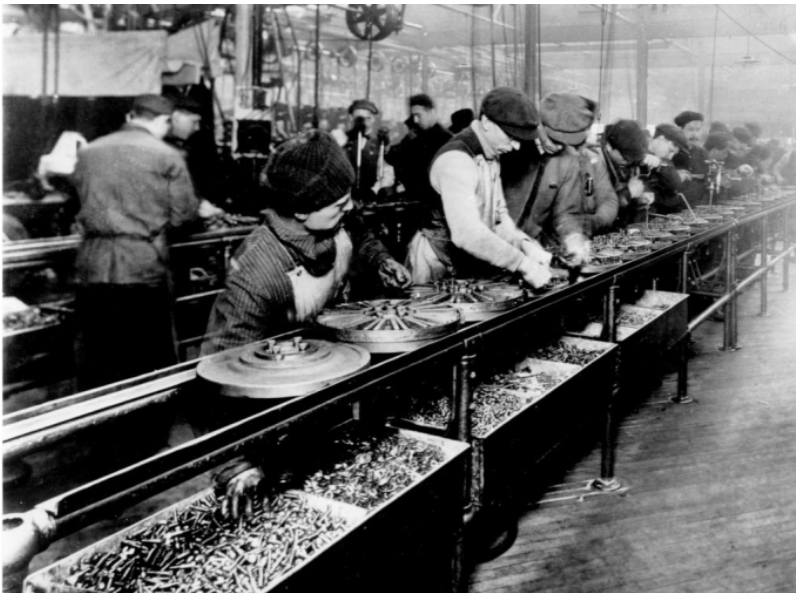
Figure 2: Workers on an assembly line at the Ford Motor Co.'s Highland Park. The use of an assembly line reduced the assembly of cars from 12 hours to 93 minutes. Retrieved from http://www.cleveland.com/business/index.ssf/2012/07/minimum_wage_hike.html
